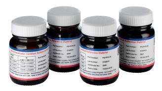
Paragon Scientific manufacture a range of Multi-Parameter Certified Reference Materials (CRMs) for refractive index and density measurements. The combined Refractive Index and Density CRM is available in four different materials, with each material including certified data for both refractive index and density at 15 °C, 20 °C and 25 °C.
